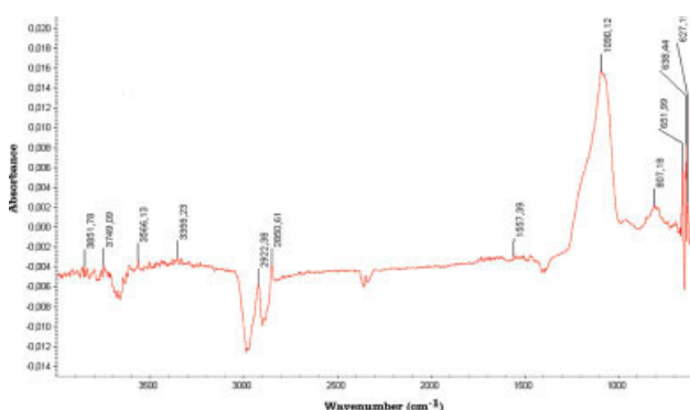
Figure A3. FTIR Spectra of sample modified with 50% of ODTCS and 20% of TMCS at 65°C at 7% RH (45 min).
